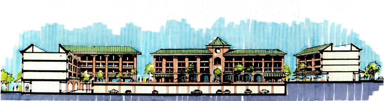
Figure 3.13: Cross-Section of Potential Redevelopment between Cooper and Centre Streets The change in grade between the new parallel connector street and the railroad station may allow for multi-story parking accessed on both levels.
